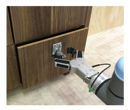
The terminal parts of the gripper are removable and allow the installation of customized elements, which we design and print in 3D so that we can fix it to the various types of samples we test.
