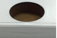
Cracks on edge (fail)
