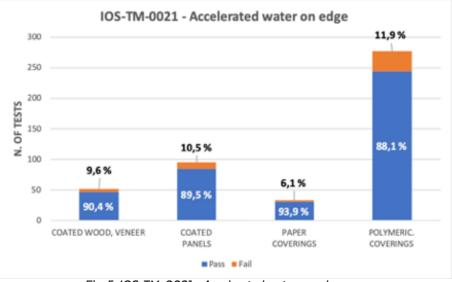
Fig. 5. IOS-TM-0021 - Accelerated water on edge.
