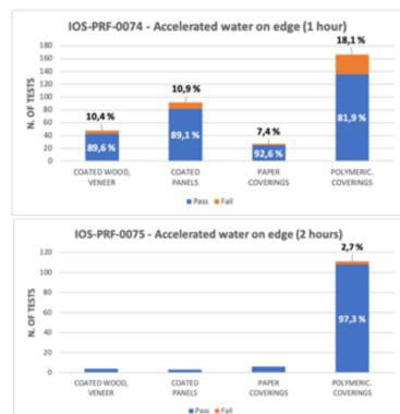
recorded for polymeric coverings (18,1 %), followed at distance by coated panels and coated woods and veneers (10,9 % and 10,4 % respectively) and finally paper coverings with a lower percentage of fails (7,4 %).
