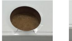
Cracks on top surface only (pass)
