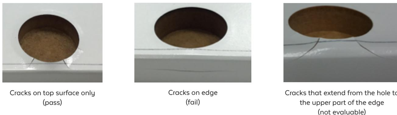
Fig. 3 - Examples of pass, fail and not evaluable cases.
