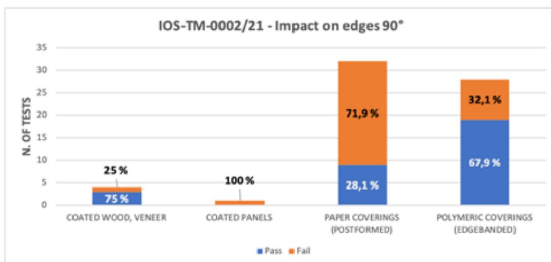
Fig. 1. IOS-TM-0002/21 - Impact on edges 90°.
