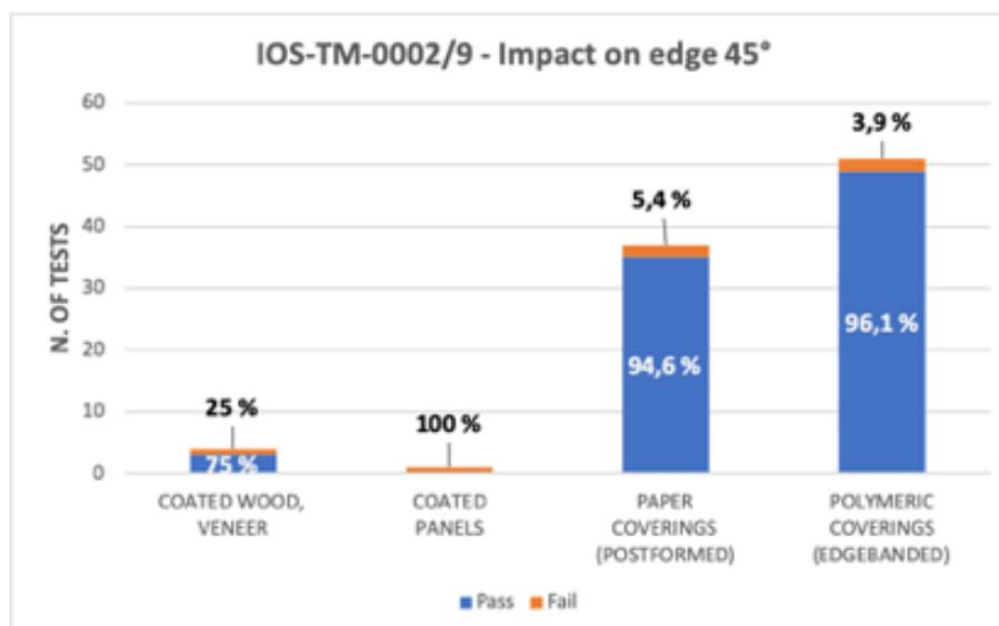
Fig. 8. IOS-TM-0002/9 - Impact on edges 45°.
