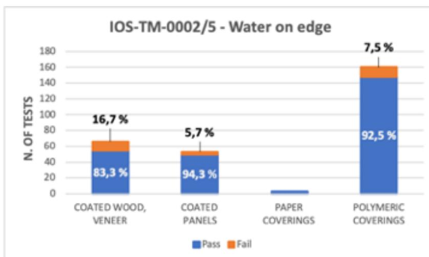
Fig. 7. IOS-TM-0002/5 - Water on edges.
