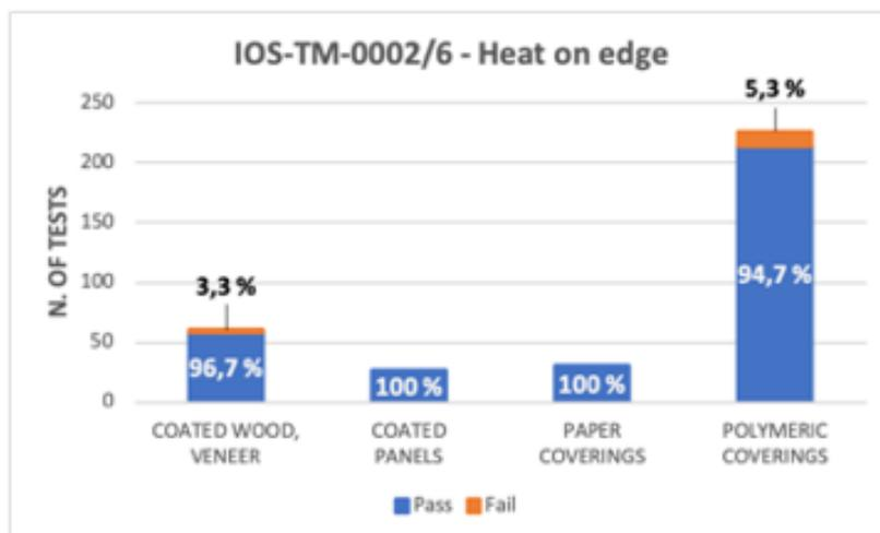
Fig. 9. IOS-TM-0002/6 - Heat on edges.
