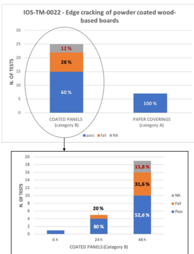
Fig. 2. IOS-TM-0022 - Edges resistance to swelling and cracking for MDF boards.
