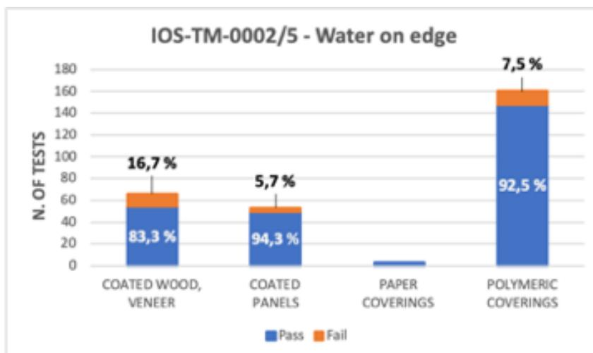
Fig. 7. IOS-TM-0002/5 - Water on edges.
