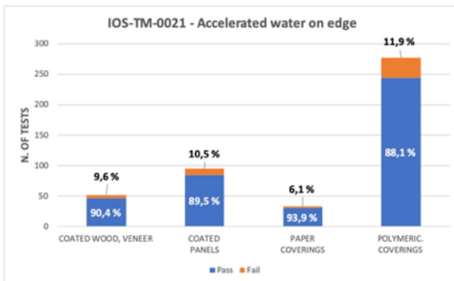
Fig. 5. IOS-TM-0021 - Accelerated water on edge.
