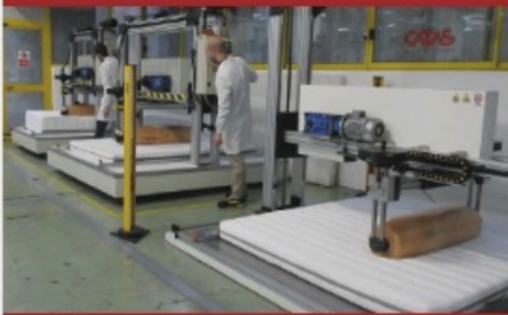
Dedicated tests on mattresses at CATAS Lissone
