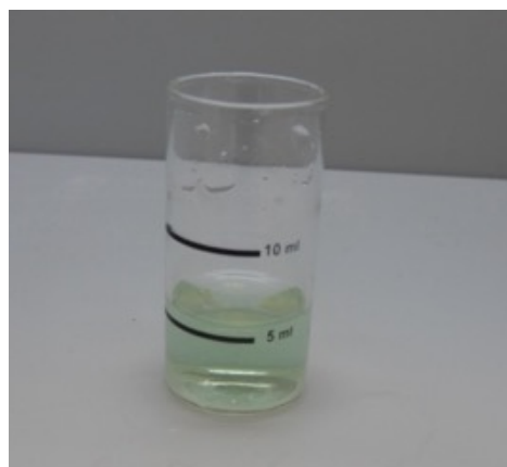
Picture 3. Water leaving the softening plant - hardness 0°HF
