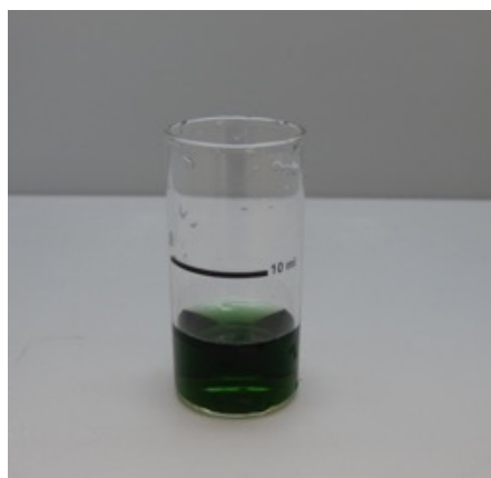
Picture 2. Water coming from the aqueduct - hardness 26°HF
