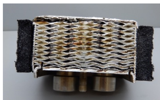
Picture 5. Limescale incrustations occurred in a heat exchanger at an operating temperature of 55°C
