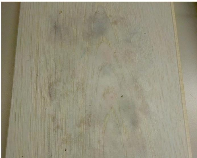
heating accelerates the drying processes, its effects can also be to promote the migration of the solvents mentioned and to soften the paint film at least initially.
