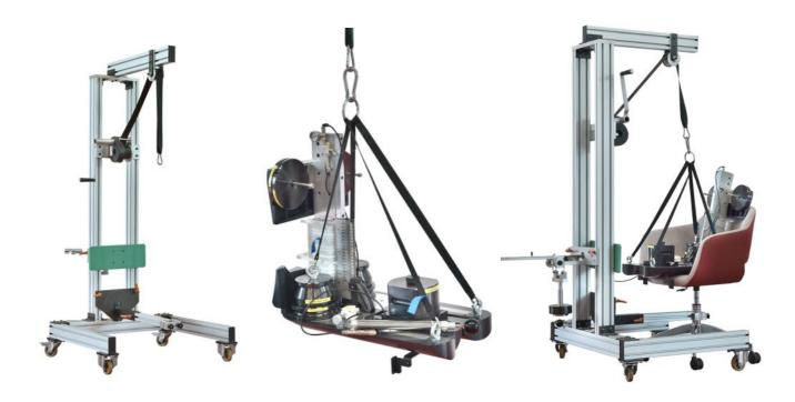
The Chair Measuring Device is built in accordance to the specifications of ISO 24496:2017 Office chairs: Methods for the determination of the dimensions and complies with the requirements of EN 1335-1:2020 Office work chairs - Part 1: Dimensions - Determination of the dimensions.
