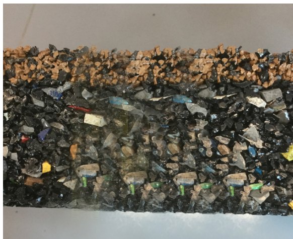
Example of rubber surface (section)
