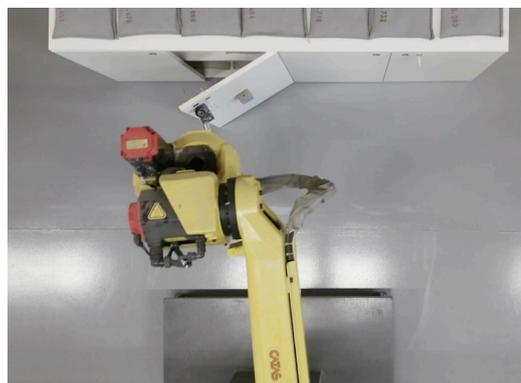
When we talk about hinges on vertical axis, hinge manufacturers can apply the **EN 15570:2008 “Hardware for furniture - Strength and durability of hinges and their components - Hinges pivoting on a vertical axis”**.
