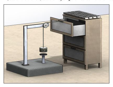
Picture 1: drawer impact with the masses method
