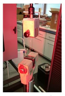
The test has been focused on two parameters: the elongation at break (as percentage) and the elasticity modulus (called also Young modulus in MPa, being the ratio of strain and deformation).
