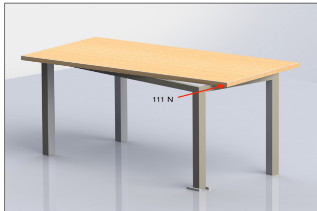
Fig.6: Unattached table top retention test Clause 25
