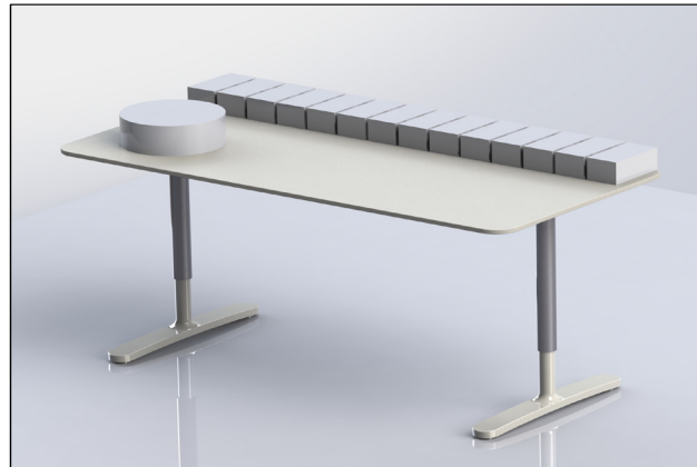
Fig.5: Work surface vertical adjustment test Clause 15
