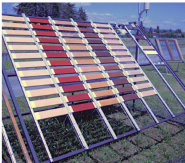
Picture 1. Natural exposure according to EN 927-3
