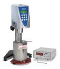
Figure 8. Brookfield rotational viscometer with heating unit
