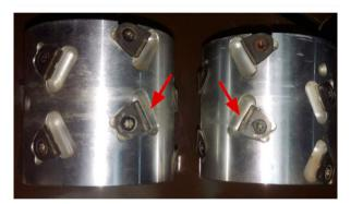
Figure 72. Example of worn premilling tools
