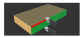
As a negative effect, the edge scraper knife tends to "whiten" the edge during cutting (working flush with the panel).
