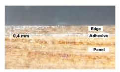
Figure 66. Insufficient pressure, adhesive line not closedFigure 67. Correct pressure, adhesive line closed
