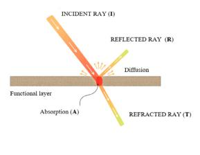
Figure 36. Schematic of the interaction between laser beam and edge
