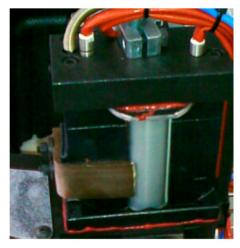
Figure 62. Correctly fed applicator roller
