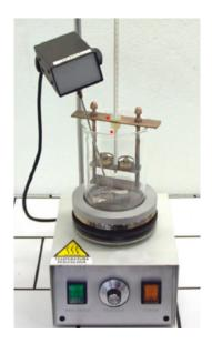
Figure 9. Instrument for determining the softening temperature of hot melts (Ring&Ball)
