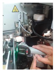
Figure 60. Infrared thermometer on the applicator roller
