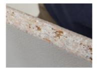
Figure 71. Example of a delaminated functional layer
