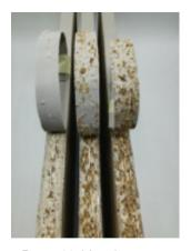
Figure 38. Visual assessment of the gluing: not sufficient (left), sufficient (centre), adeguate (right)
