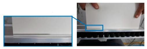
Figure 78. Example of rectified panel with not aligned cutters
