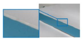
Figure 82. Example of profile irregularities due to chips under the vertical tracer
