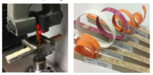
Figure 43. The peeling testFigure 44. Plastic edges after the peeling test
