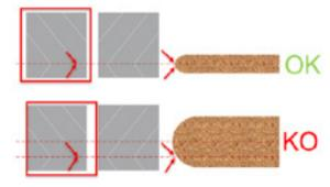
Figure 31. Asymmetrical tools on postformed panels
