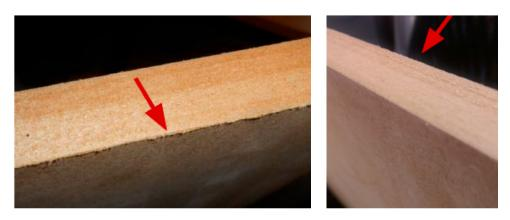
Figure 73. Example of a panel with a damaged cut line due to a worn tool
