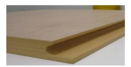
Figure 18. Shaped MDF panel (JPull type) for soft forming application
