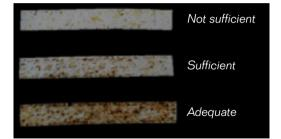
Figure 40. Visual assessment of the removed wood particles after the peeling test
