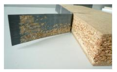
Figure 65. Example of an incorrect gluing with applicator roller not properly squared
