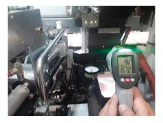
Figure 53. Infrared thermometer on the adhesive head
