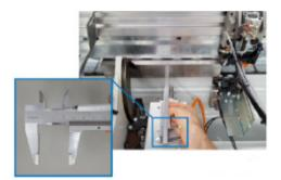
Figure 79. Example of measurement of the working line: distance between the side surface of the panel and the track support measured with the caliper
