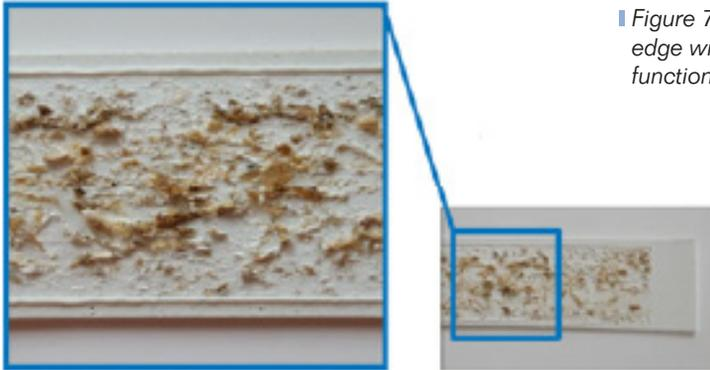
Figure 70. Example of an edge with a correctly cast functional layer
