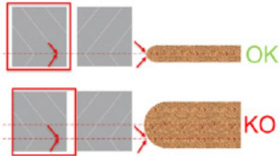
Figure 31. Asymmetrical tools on postformed panels
