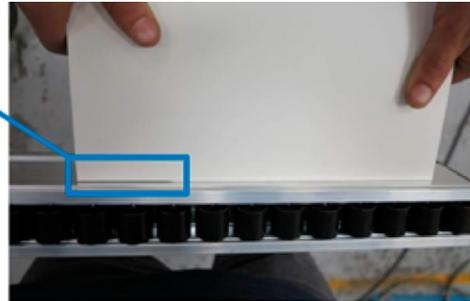
Figure 78. Example of rectified panel with not aligned cutters
