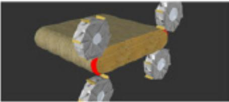
The unit carries out a finishing process with edges in coils. The corner rounding unit can consist of one, two or four motors with dedicated cutters that remove material at the four corners of the panel, in the area of the sharp edge of the tape which is therefore rounded at the end of the processing.
