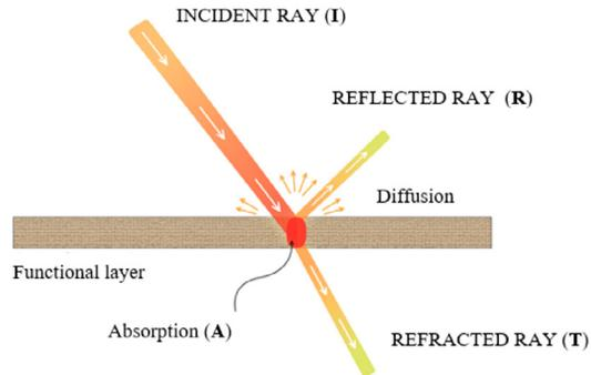
Figure 36. Schematic of the interaction between laser beam and edge
