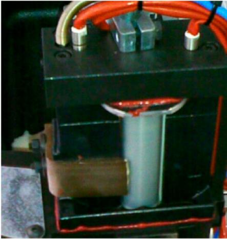
Figure 62. Correctly fed applicator roller
