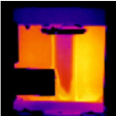
Figure 63. Thermal image of an applicator roller with incorrect software parameters or a non-functioning heating elements
