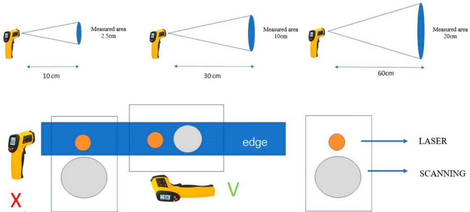
Figure 54. Procedure for using a laser pointer thermometer
