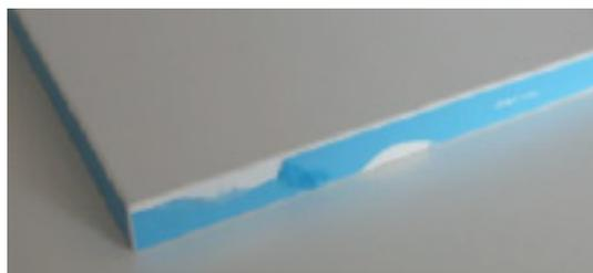
Figure 83. Example of edge with the protective film removed from the front copiers of the corner rounder
