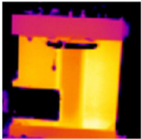
Figure 64. Thermographic image of a properly functioning applicator roller
