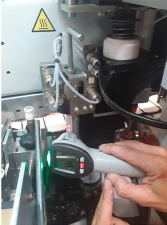
Figure 60. Infrared thermometer on the applicator roller
