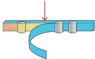
Figure 11. Position for measuring the assembling temperature
