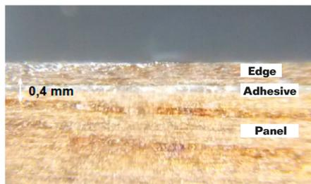
Figure 67. Correct pressure, adhesive line closed
