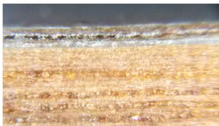
Figure 66. Insufficient pressure, adhesive line not closed
