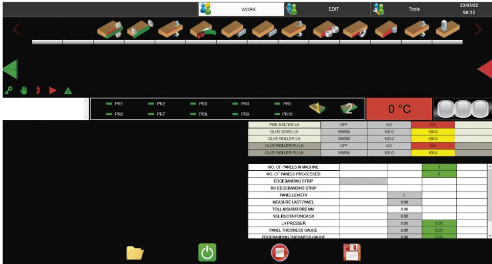
Figure 59. Edgebander control panel
