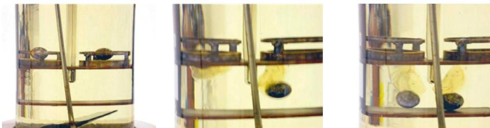
Figure 10. Test for the determination of the softening temperature
