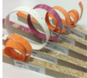
Figure 44. Plastic edges after the peeling test
