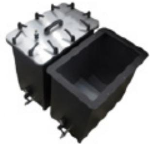
Figure 69. Nitrogen tank to inhibit the cross-linking of the adhesive
