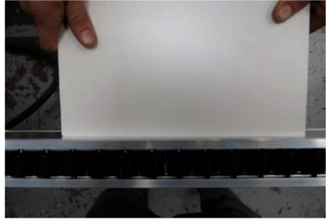
Figure 77. Example of premilled panel with perfectly aligned cutters
