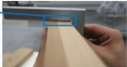
Figure 76. Example of a 45 mm thick panel premilled with non-squared cutters
