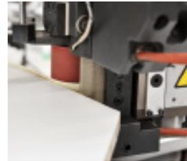
Figure 20. CNC edgebanding process
