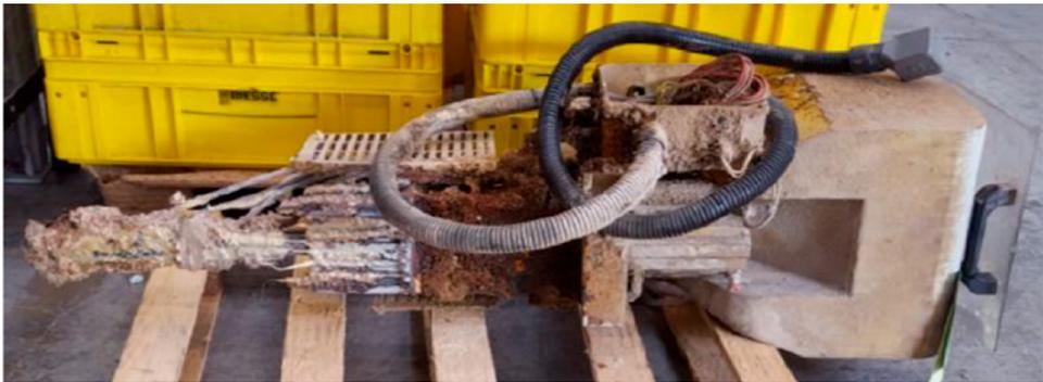
Figure 49. Example of an uncleaned premelter
