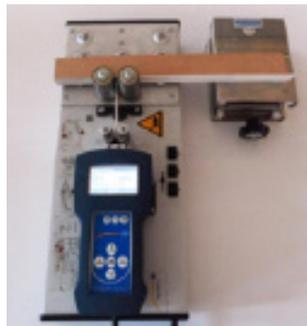
Figure 39. Portable dynamometer for the peeling test
