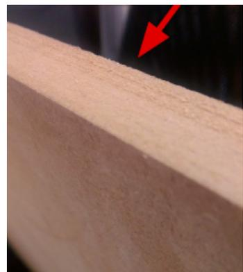
Figure 73. Example of a panel with a damaged cut line due to a worn tool
