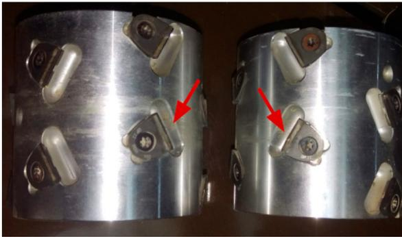
Figure 72. Example of worn premilling tools
