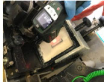
■ Figure 56. Infrared thermometer for surface temperature control (not suitable for depth checks)
