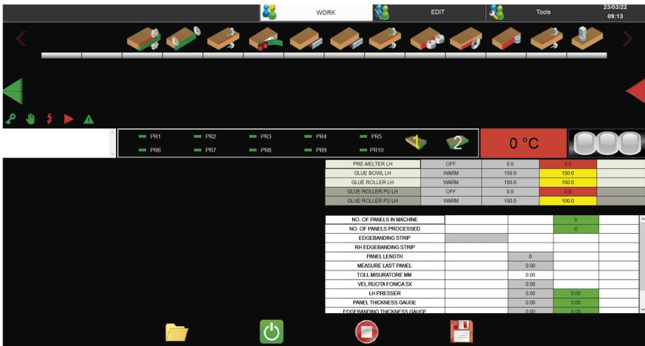
Figure 52. Melting parameters on the control of the edgebander
