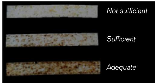
Figure 40. Visual assessment of the removed wood particles after the peeling test
