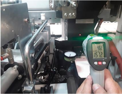
Figure 53. Infrared thermometer on the adhesive head
