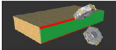
The fine trimming unit consists of two motors with specific tools capable of removing the top and bottom edge excess. The quantity of residual material must be the optimal one, that is 0.2 mm, for the subsequent processing carried out by the edge scraper unit.
