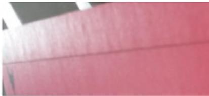
Figure 74. Orange peel effect
