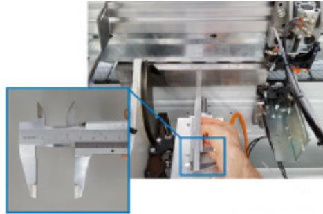
Figure 79. Example of measurement of the working line: distance between the side surface of the panel and the track support measured with the caliper
