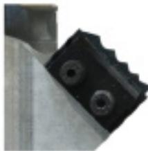
Figure 81. Example of a perfectly worked edge without “beats”
