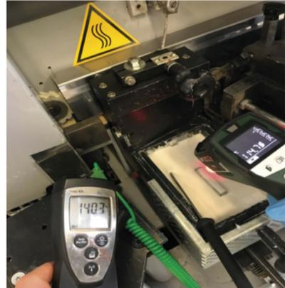
Figure 58. Detected temperature: difference between immersion thermometer and infrared thermometer
