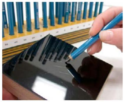
Figure 4.2 Hardness by pencil test
