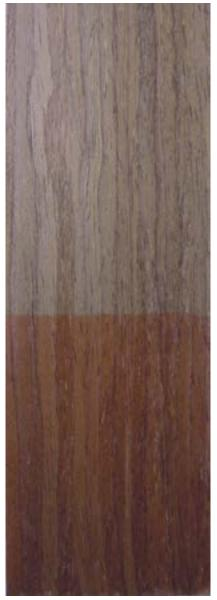
The upper part was exposed to light, whilst the lower surface was protected as reference.
