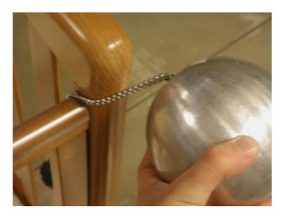
The major changes are in **clause 4.4.8.2**. The standard describes how to measure the height between any foothold or base mattress and the top of sides and ends.
