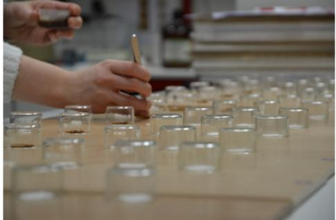
These pictures show the cold liquid resistance tests performed at Catas during the long phase of standard setup. The study involving six Italian coating producers was used to establish the minimum requirements then inserted in the UNI 11622-1.
