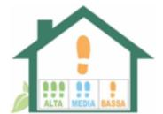
The labels reported by UNI 11622 are simple images of a house with one, two or three footprints. They can be used to immediately identify the coating suitable for the specified environment.
