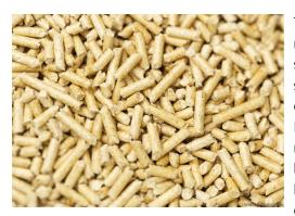
The production of pellet is based on the compacting process of powder wood materials in order to get a homogeneous product with relevant advantages such as obtaining a standard, easily preservable, stockpileable, easy transportable product that enable regular combustion with high energy yields and reduced emissions.
