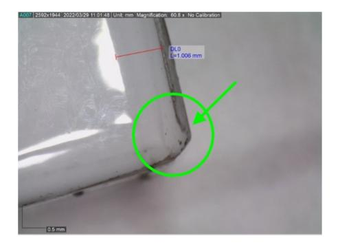
The red line that is above the green circle show the thickness measure, which is 1.0 mm. This is exactly why the edge is **NOT sharp** (see results of the hazard perception survey).
