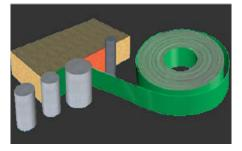
Step 5: the working station carries out a rough trimming process in the case of the application of roll edges and a finishing process in the case of solid wood edges. The trimming unit consists of two horizontal motors equipped with specific tools capable of removing the excess of the upper and lower edge.
