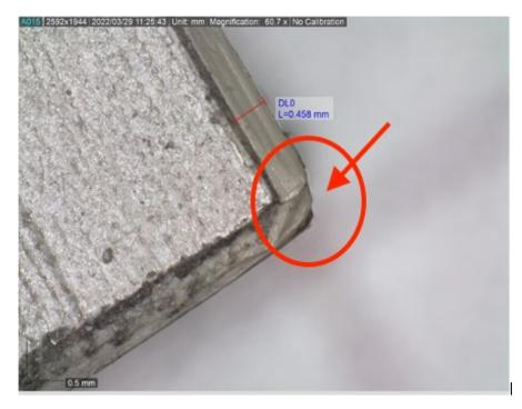
Confirming what said before above, the thickness of the edge applied on the panel is 0.4 mm.
