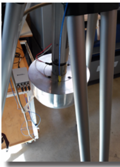
Fig. 1: Equipment for determining the critical fall height.
